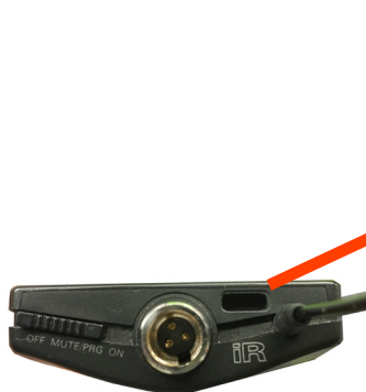
PT450/PT470 – The IR Sensor is located between the antenna and mini XLR Jack
