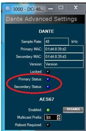
When connected, status is blue. When disconnected, status is dark.
