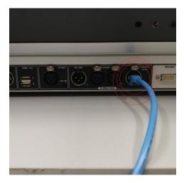
From Control Surface (Control Data Port) > Front of Active Breakout Box (Control Data Port)
