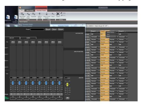
This provides a simulation where controls will move to reflect the parameter values stored in the Parameter Preset.
