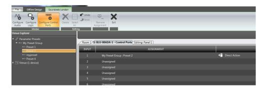
• The Control port is updated to reflect the Direct Action assignment. When the Configuration is loaded to the device, the Parameter Preset will be recalled when the Control Input pin is shorted with the Common pin.
