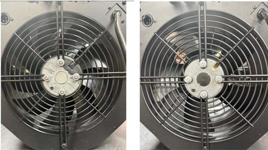
Any 230V unit after serial I4509793701 (production date 1st March 2023) or any 115V unit after serial I4509794101 (production date 3rd April 2023) will have the new 5 blade fan installed.
