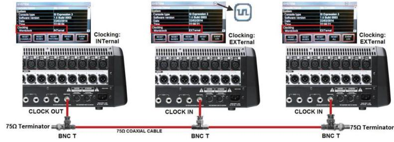
Use an external generator to distribute word clock to each console. Set BLU-SI option card as instructed above. All consoles will be deriving their word clock from an external source. These must have the Wordclock set to EXTERNAL.
