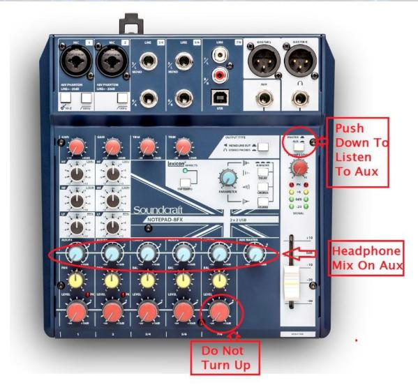
Note- The Aux Bus sum is sent to the Aux Master output level control. This sum is made up of the aux send pre-fade contributions from each channel. That is, the sends are taken before the input channel fader and are not affected by the input channel fader levels. So your headphone mix is totally independent of the L&R mix going to your computer. You can listen back and forth by selecting either L&R or Aux on the headphone mix select button
