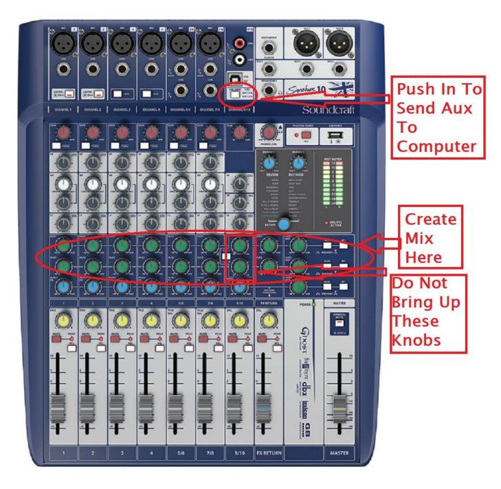
Note- Select Post Fade for the Aux so the levels of the mic faders are also what you are sending to the aux, thus to the computer. Set the knobs for each channel in the Aux mix at the mark at 2 o'clock
