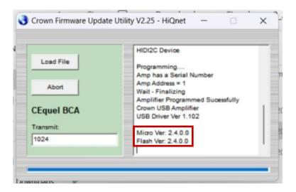
The firmware update process is now complete. **Be sure to use Audio Architect v2.55.2.2 or later** when trying to connect your XTi series amplifier for configuring. It will not work with previous versions.
