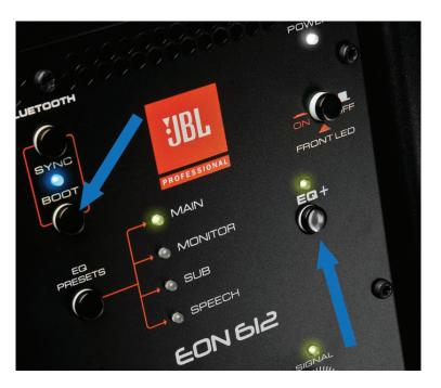
Press the SYNC button To broadcast the Bluetooth address.
