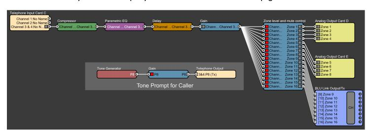
This feeds a Matrix Router that is controlled via Parameter Presets to route the page to the desired output. A single output Crossover is on each output to provide a gain & mute point as well as some High and Low pass filters commonly required in distributed audio systems.
