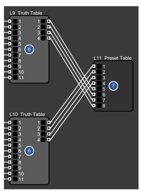
The last action of the circuit is to reset the router when the Hybrid card goes on hook at the conclusion of the page. When the Hybrid goes On Hook, all counters reset and the Snapshot objects go into Bypass; clearing the router and preparing the logic circuit for the next page.
