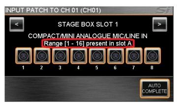
4. The MADI USB channels (to and from computer) start at 33. This is the mixer's internal buss channel number and NOT the channel number that will show in computer. In this example, MADI channel 33 is selected and this will show up as channel 1 in computer.
