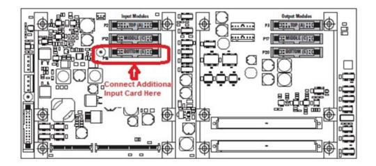
The 3 module slots are labeled A, C and E; they correspond to the connectors of the backplane PCB according to the illustration above. There are 3 connectors on the left for input modules, and 3 on the right for output modules. Modules must be connected to the correct connector in order to have a correct assignment of input and/or output channels.
