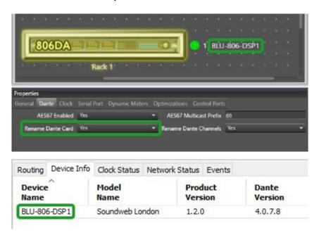
The Device Name entered in Audio Architect will be pushed to the Dante card if the Rename Dante Card property is set to Yes. This is the default setting. It will not be possible to rename the Dante Device Name using Dante Controller with this setting.
