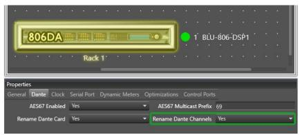
The Dante channel label will comprise the Object Name and Channel Name separated with a hyphen (-)
