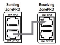
• The cable length of the linking cable must not exceed 25' Linking more than 3 ZonePROs is typically not recommended, as systems of this size generally require processors with a more sophisticated feature set.
