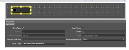
The serial messages are entered in the Serial Table field by clicking the Click to edit Serial Table/Trigger button.
