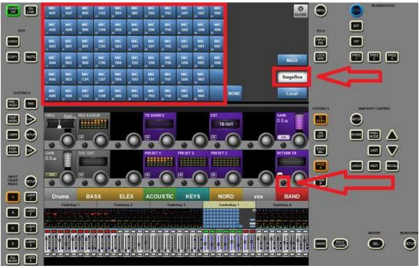
6. To patch TB Return to an output, use the **MONITORING SETUP** page. Since both the FOH & Foldback consoles are tied to the MADI stagebox channels, either or both consoles can monitor RETURN TB from the stage. In this example, I have patched RETURN TB to both MONITOR A & HEADPHONES for versatility. But, this can be assigned to just one or all three monitoring solutions.
