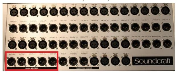
9. For the Vi1, Vi2, 1000, 2000, or 3000, the monitoring outputs will need to be assigned to a local output channel at the back of the console, if not already assigned.
