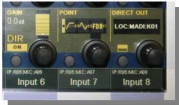
Si channel patched to a Vi Stagebox
