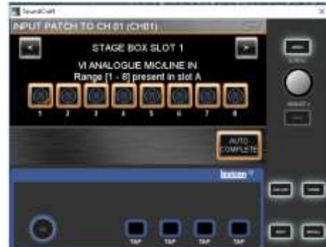
Si Patch screen showing patching to a Vi stage box mic card
