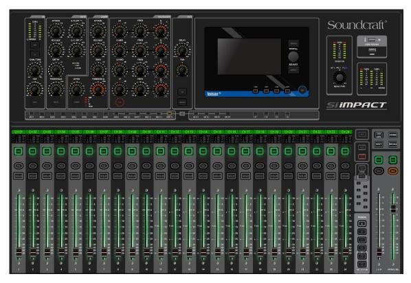
If you run into this issue, here's how to resolve. Select that channel and Select Input on screen. Scroll down to the affected mix in the Per Mix Post/Pre section. Scroll to All Pre Dyn and select by pushing down on encoder.
