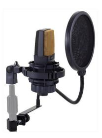
Popping sounds occur particularly in the pronunciation of aspirated plosives (such as the first 'p' in the English word "popping"). The popping sound recorded by a microphone has two components: High-frequency components are from air moving past the grille or other parts of the microphone body. The low-frequency component is from air impacting the diaphragm. Mechanical and electrical saturation (e.g. clipping) can also play a role depending on the amount of headroom designed into these systems.
