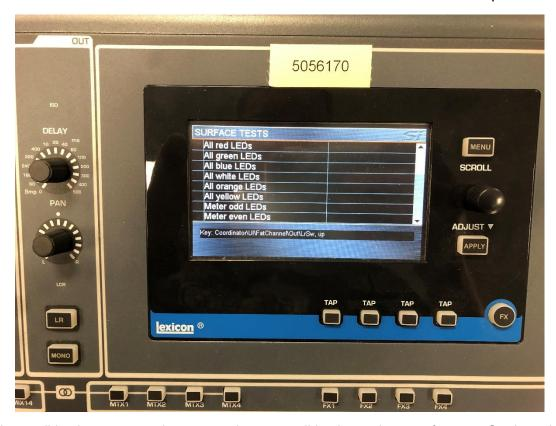
Use the scroll knob to move in the menu and press scroll knob to select test function. Go through the list and check each function. In the surface test, there are two key checks: the all LEDs ON and fader position test. All LEDs ON will show you if any LEDs have gone bad. The fader position test will show if any faders are not moving or moving slowly compared to the rest. These faders will need to be replaced.
