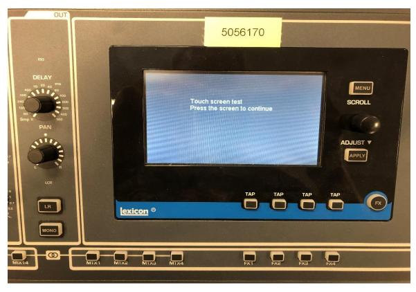
Touch screen test: Tap touch screen and follow the white button on the screen, keep tapping the screen as the display goes through different patterns & colors. (Last screen is the vertical color lines)
