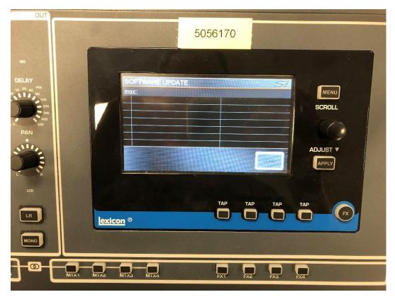
Press and hold LR and MONO button and tap the FXI button, once. Then repeat, press and hold LR and MONO button and tap the FXI button to see the Format SD Card button on the display. Tapping to this option is going to clear the SD card. Clearing SD Card will erase all shows and passwords for all user accounts!
