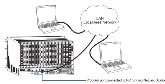
FIG. 27 Enova DGX 32 connected via a LAN to two PCs (Program port is connected for initial set up)
