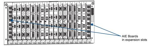
FIG. 70 AIE Boards (shown with HDMI Input and Output Boards in Enova DGX 32)
