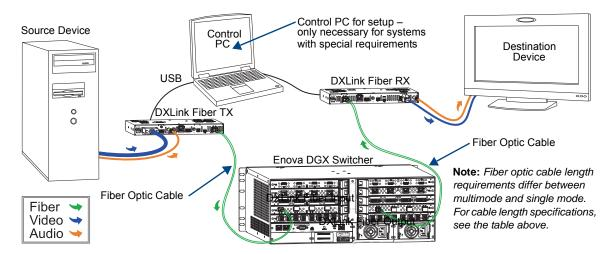
FIG. 54 DXLink Fiber Boards are used in conjunction with DXLink Fiber units
