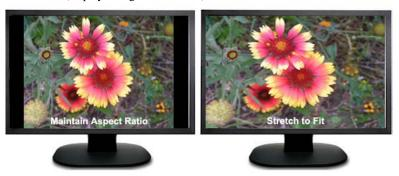
FIG. 107 Example of displays set to Maintain Aspect Ratio and Stretch to Fit
