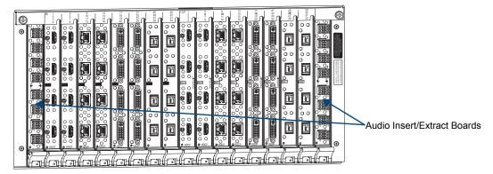
FIG. 22 Audio Insert/Extract Boards in an Enova DGX 32
