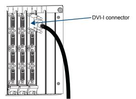
FIG. 43 Fasten cables onto input and output connectors
