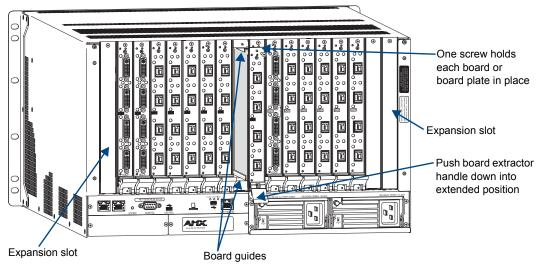
FIG. 129 Enova DGX 32 - Remove screw, push board extractor handle down, and then pull board straight out
