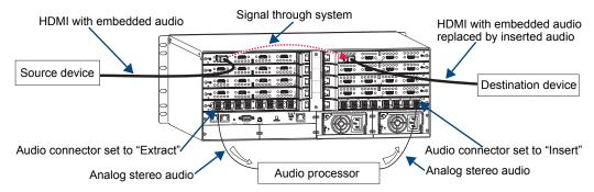
FIG. 75 Audio extracted from HDMI input signal and inserted onto HDMI output signal(s)
