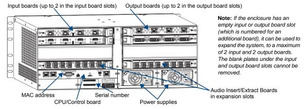
FIG. 3 Rear view of a fully loaded Enova DGX 8 enclosure with two expansion boards
