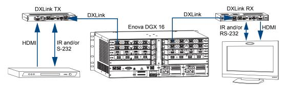
FIG. 52 Serial data transfer and IR flow control
