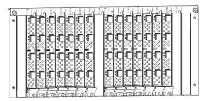
FIG. 53 DXLink Fiber Boards, Simplex and Duplex (shown in Enova DGX 32 with dust plugs)
