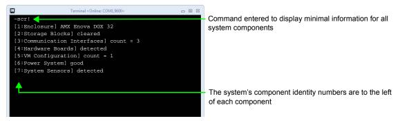
FIG. 120 Example of a default Enova DGX 32 splash screen
