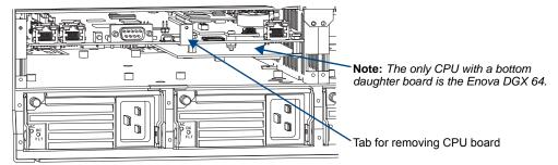
FIG. 140 Use tab to pull CPU board straight out (Enova DGX 64 shown)
