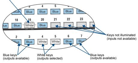
FIG. 84 Example of key states during Change Mode (Control Panel on an Enova DGX 32)
