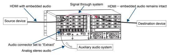
FIG. 71 Audio extracted from HDMI input signal and sent to auxiliary audio system
