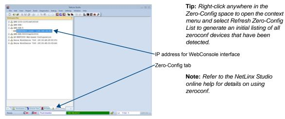
FIG. 33 NetLinx Studio showing the Zero-Config tab and the IP address for a WebConsole interface
