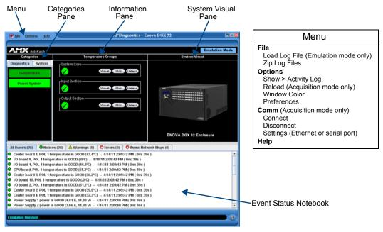
FIG. 119 Main screen in Emulation mode (the Comm menu option is not available in this mode)
