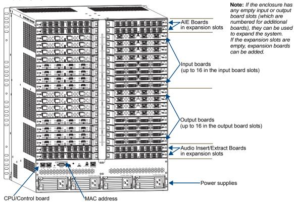
FIG. 6 Rear view of a fully loaded Enova DGX 64 enclosure with eight expansion boards
