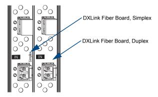
FIG. 57 DXLink Fiber Boards, Simplex and Duplex
