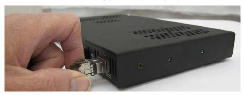
FIG. 65 Pull transceiver free from transceiver socket
