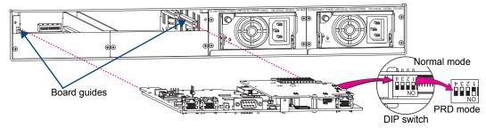
FIG. 137 Set Position #1 DIP switch to ON for NI Series
