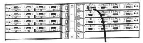
FIG. 41 Attach HDMI connectors to HDMI receptacles
