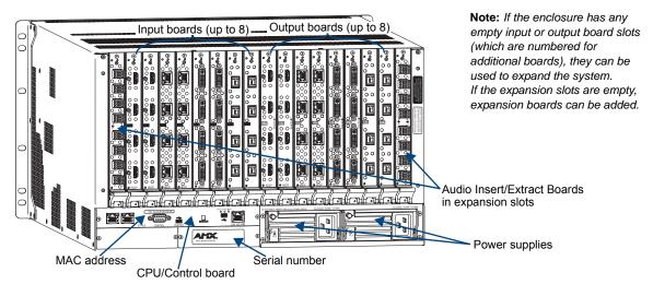
FIG. 5 Rear view of a fully loaded Enova DGX 32 enclosure with two expansion boards
