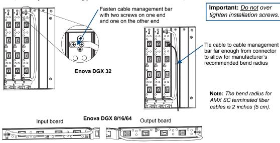
Note: On the Enova DGX 8/16/64, the orientation of the cable management bar is reversed from input to output board.
