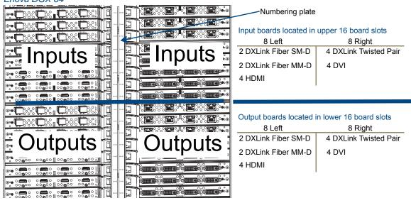
FIG. 12 HDMI, DVI, DXLink Twisted Pair, and DXLink Fiber Input and Output Boards shown
