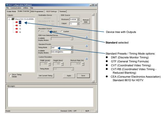
FIG. 110 Scaler Override view with Standard Presets selected
