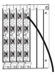
FIG. 50 Fasten cables onto input and output connectors
