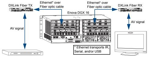
FIG. 60 Serial data transfer and IR flow control with Duplex hardware in Bidirectional Mode
