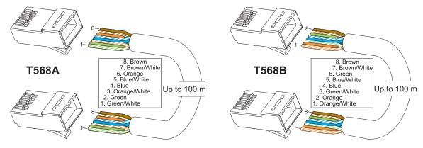
FIG. 49 Twisted pair cable pinouts for T568A and T568B
