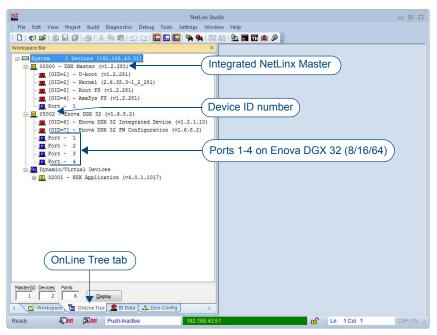
FIG. 104 NetLinx Studio OnLine Tree - indicating Master number and device number and ports for Enova DGX
