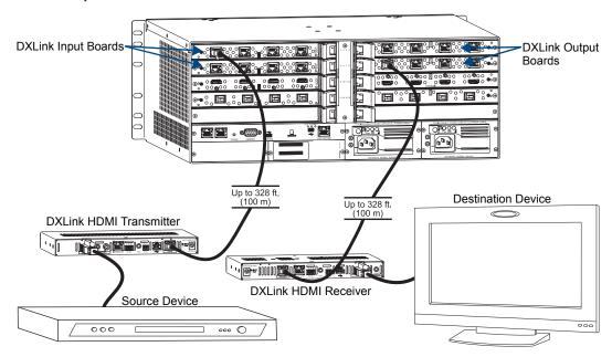
FIG. 46 DXLink Boards used in conjunction with DXLink Transmitter and Receiver
