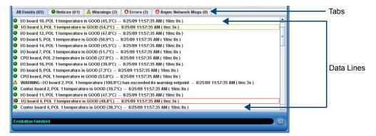
**Note:** A yellow or red outline around a data line indicates that the component was previously in a Warning or Error state.
