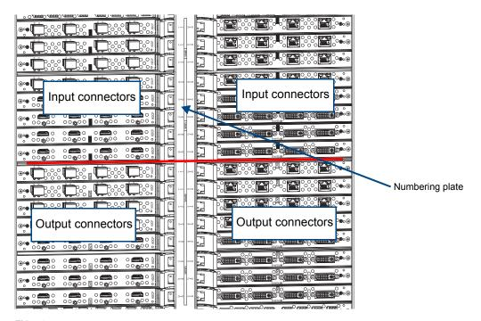
FIG. 21 Numbers on numbering plate indicate input and output board channels
