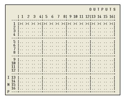
FIG. 143 DGX\_SHELL switch command displays matrix switching status in a table (Enova DGX 16 shown)
