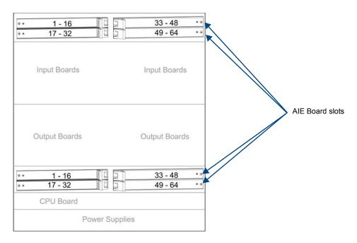
FIG. 79 AIE Board slot numbering on Enova DGX 64
