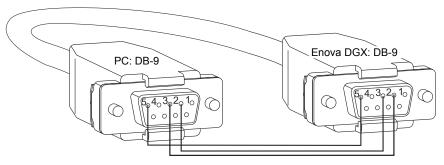
FIG. 35 RS-232 null modem cable pin diagram, no hardware flow control
