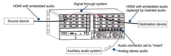
FIG. 73 Audio inserted onto HDMI output signal
