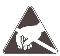
To avoid ESD (Electrostatic Discharge) damage to sensitive components, make sure you are properly grounded before touching any internal materials.
