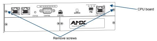
FIG. 135 Remove screws indicated
