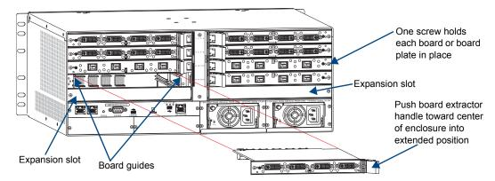
FIG. 130 Enova DGX 8 (16/64) - Remove screw, push extractor handle right (input) or left (output), pull board straight out
