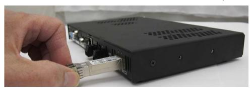
FIG. 66 Insert transceiver into transceiver socket
