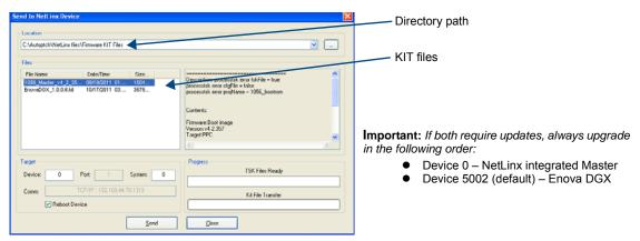
FIG. 103 Send To NetLinx Device dialog showing KIT file for the integrated Master selected
