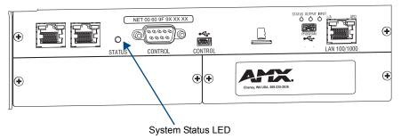
FIG. 138 Check System Status LED indicator
