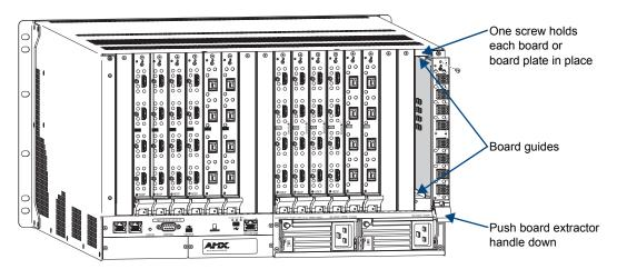
FIG. 77 Remove screw, push board extractor handle down, then pull board straight out (Enova DGX 32 shown)
