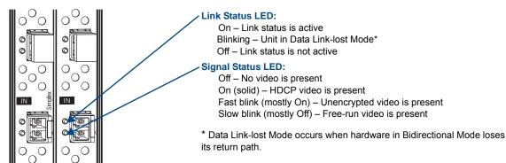
FIG. 58 Fiber optic transceiver LEDs on Duplex Input Board
