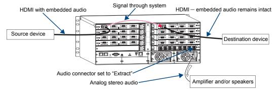
FIG. 74 Audio extracted from HDMI output signal
