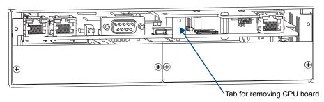
FIG. 136 Use tab to pull CPU board straight out
