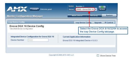
FIG. 90 icsp Device Config tab/page – Enova DGX 16 Device Config
