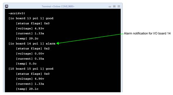
FIG. 132 Terminal information showing an "alarm" for a board that has not powered up correctly
