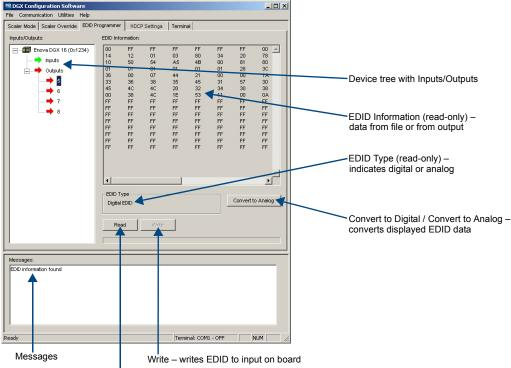
Read – reads EDID from selected output which received the EDID from its attached destination device
