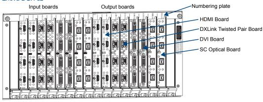
FIG. 11 HDMI, DXLink Twisted Pair, DVI, and SC Optical Input and Output Boards shown
