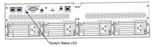
FIG. 142 Check System Status LED indicator (Enova DGX 64 shown)
