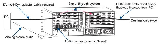
FIG. 72 Audio inserted onto HDMI input signal
