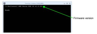
FIG. 121 Power-up splash screen in DGX Configuration Software's Terminal view
