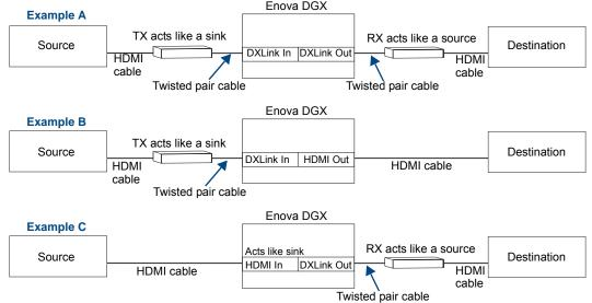
Example A: When a Receiver acts like a source, its key does not count. Source device sees 1 key (Transmitter).
