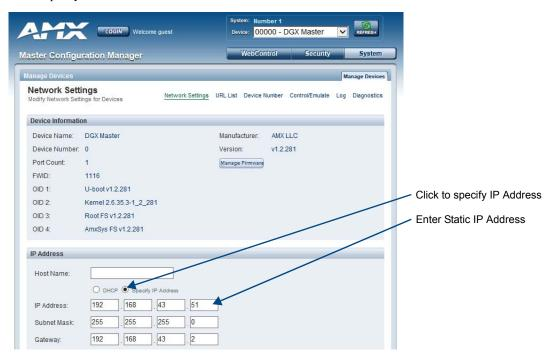
FIG. 89 Network Settings page with static IP Address
