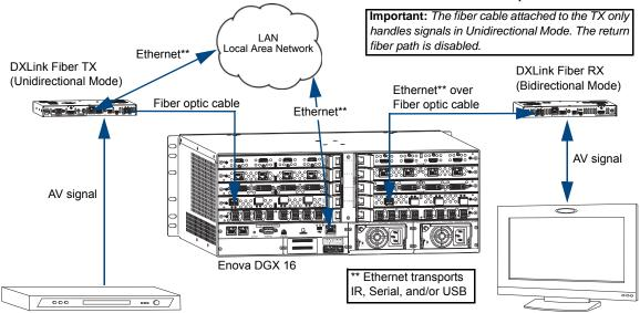
FIG. 61 Serial data transfer and IR flow control with TX in Unidirectional mode and RX in Bidirectional Mode
