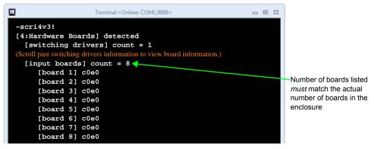
FIG. 131 Splash screen showing boards in the system (Enova DGX 32 example with 8 input boards)
