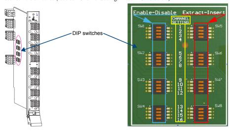
FIG. 78 Flip DIP switches to change settings
