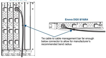
FIG. 56 Attach cables to input and output connectors (shown with cable management bar)
