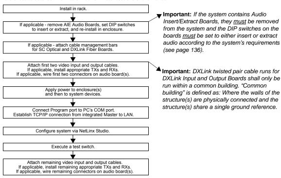
FIG. 15 Flow chart for installation procedure
