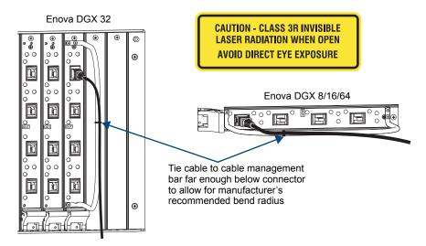
FIG. 69 Fasten cables onto input and output connectors (shown with cable management bar)
