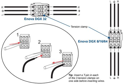
FIG. 80 Audio wiring for AIE Board
