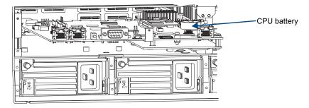
FIG. 141 Locate CPU battery in battery bracket (Enova DGX 64 shown)
