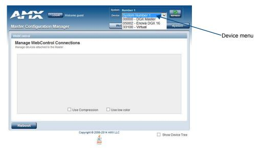
FIG. 86 Device menu in the Master Configuration Manager
