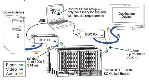
FIG. 68 SC Optical Boards are used in conjunction with DGX Fiber Modules
