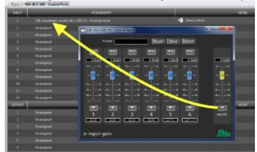
In the Mode column there are four options - Direct Action, Direct Action (inverted), Toggle Action and Mutli-State. You will use Direct Action or Direct Action (inverted) depending on whether the closure from the Fire Alarm system is normally open or normally closed.
