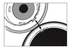
5. While holding the earpad in place with one hand, use the mounting tool to firmly press the inner part of the earpad until the hooks snap in place.
