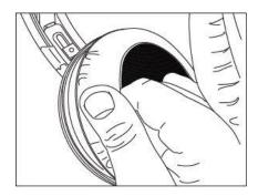
2. Make sure the sealing gasket is in place on the speaker plate.
