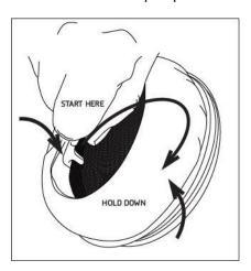
6. Moving clockwise around the earpad, use the mounting tool to press each clip into place. Proceed around the inner side of the pad until all hooks are snapped in.
