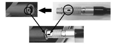
2. To disconnect please pull the metal moving part on the connector, which causes the pins to retract into the housing, releasing the bond.
