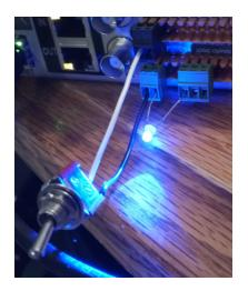
In the picture above you see a double pole single throw [DPST] switch connected to Control Input I, and an LED connected to Control Output I. The LED is polarized, meaning it will only light if the correct voltage is applied in the correct direction.
