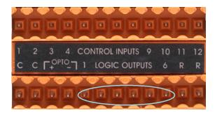
These ports can be set up in two or three wire mode which we will cover shortly. By default the configuration is two-wire mode meaning that inputs or outputs are connected between the appropriate pin specified in the design and one of the two common connections at the bottom on the left.
