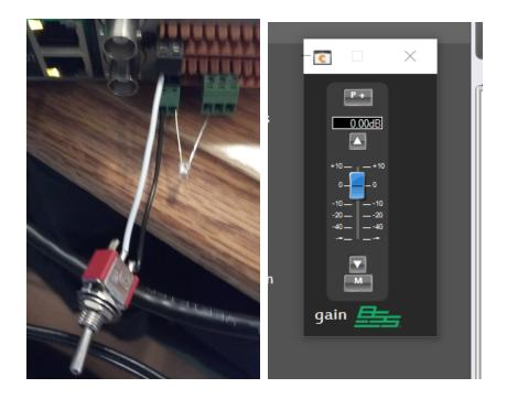
If the switch is changed to the closed state, the mute and LED will turn on.
