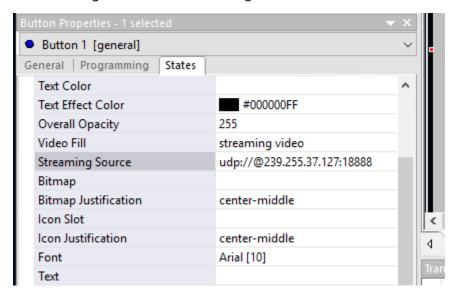
In the example above, we are using the multicast stream output by the encoder.
