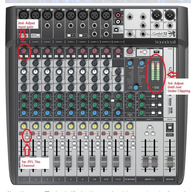
Notepad has no way to PFL a channel so I found a quick way to get best gain is to turn up input gain until you see the peak LED, then bump down just under clip.
