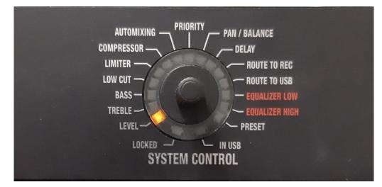
6. Now you need to speak into the microphone and set the input gain on the rear panel till you get the desired level. Don't exceed the 0 dB indicated on the front.
